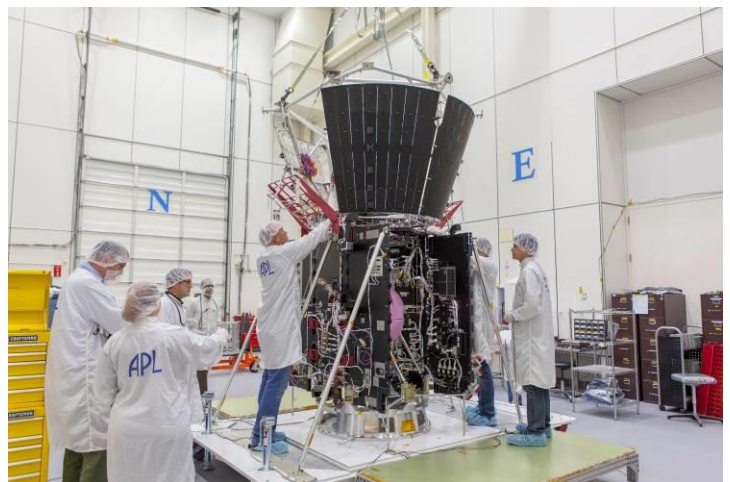
Assembly of Parker Solar Probe.
